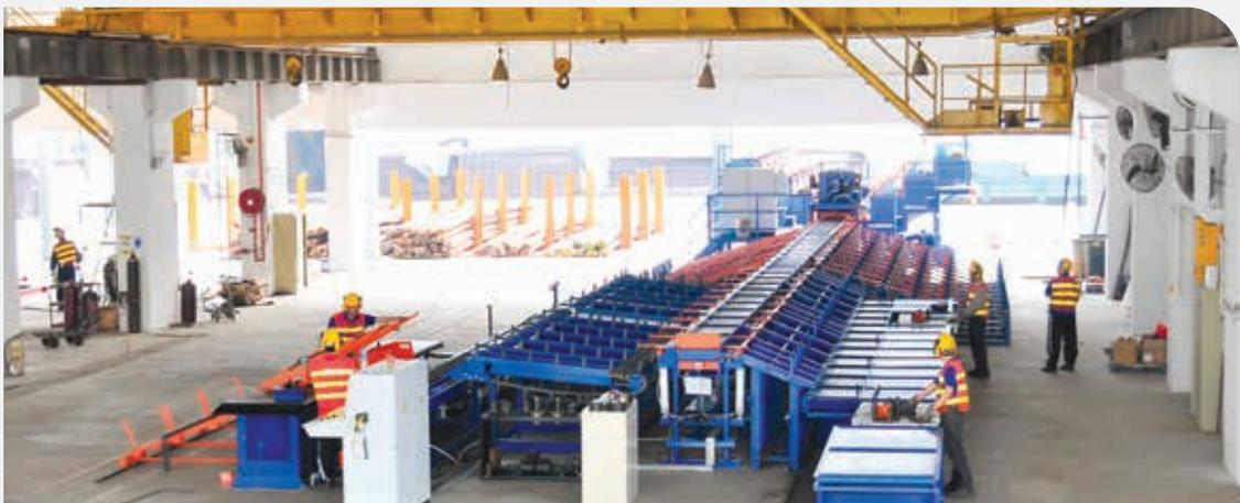
Automated Cut-and-bend Rebars Processing Plant in Tai Po, Hong Kong
